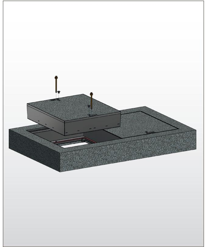
*Covers for cable and/or utility shafts in tunnel structures, square design*
